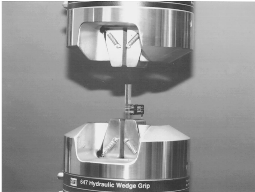
Figure 10 Photograph of the testing apparatus used for all tensile testing. Also shown is a tabbed Ceracarb™ test specimen mounted with a clip-gage extensometer.
