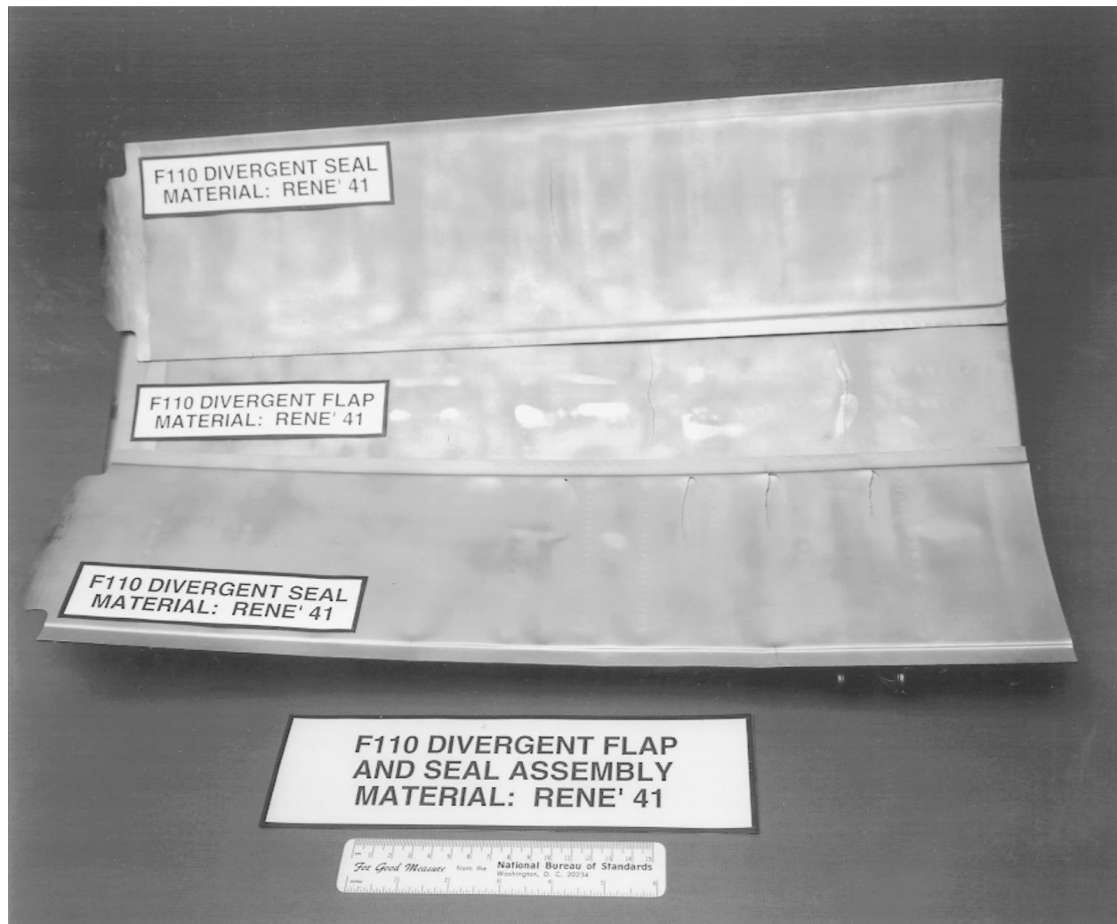
Figure 1 A photograph of a GE-F110-100 exhaust nozzle divergent flap and two divergent seals that have been removed from service due to severe cracking. The Rene'41 components suffer from extensive creep deformation and cracking due to the environment.
